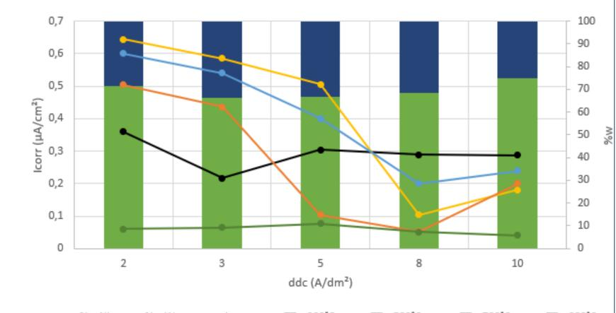
■ %w Ni ■ %w W → w/oTT → TT = 300°C → TT = 500°C → TT = 700°C → TT = 900°C
